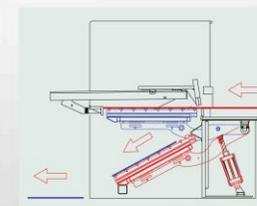
Pneumatic support system (monobloc panel type) working principle.
