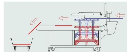
Conveyor system working principle.
