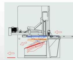
X type pneumatic sheet support system working principle.
